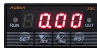
Figure 8. The display of the JSL-64A timer in ESP mode.
