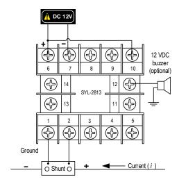
Figure 1. A wiring diagram of measuring direct current with a shunt resistor on Channel1 of a SYL-2813.
