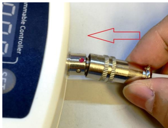
Figure 4. Install the sensor.
