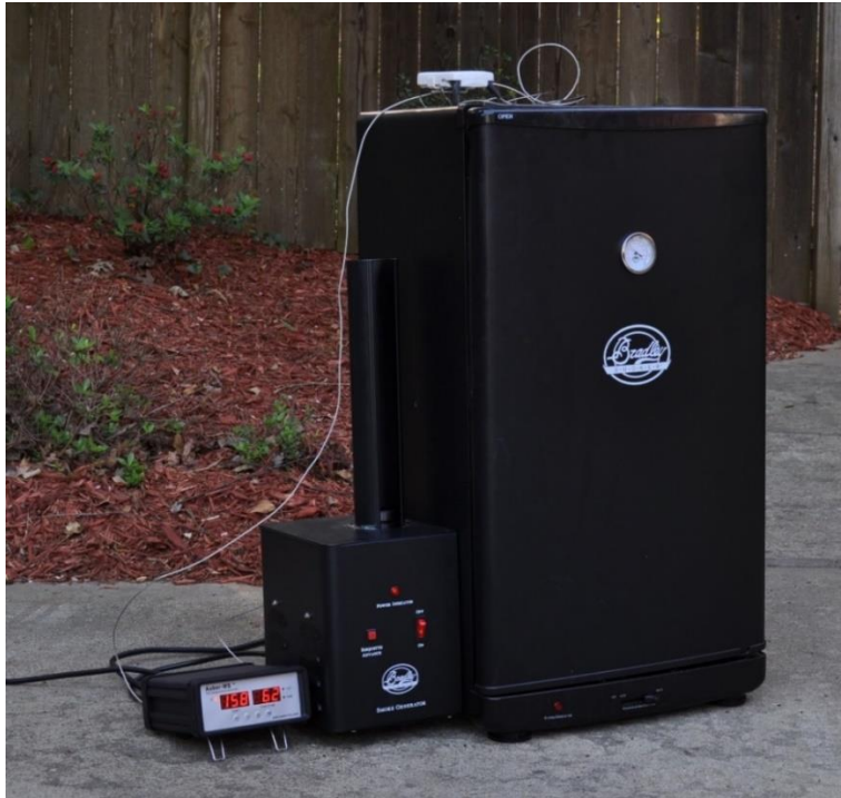
Figure 7. Connection between the controller and smoker
