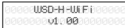
Figure 10. Initializing display. Top line is for model number. Bottom line is for firmware version.
